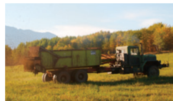
A customized, five-ton, 6x6 military truck, mounted with Loewen manure spreader, is used to conquer steep slopes in rainy conditions.
