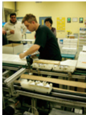
Schanck conducts the first visual inspection of the printed and coded Holstein tags as he transfers the finished tag sets to shipping nests.
